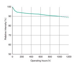
※11 Horizontal luminous intensity at continuous use. Frequent switch may cause shorter life.
