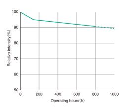
※11 Horizontal luminous intensity at continuous use. Frequent switch may cause shorter life.
